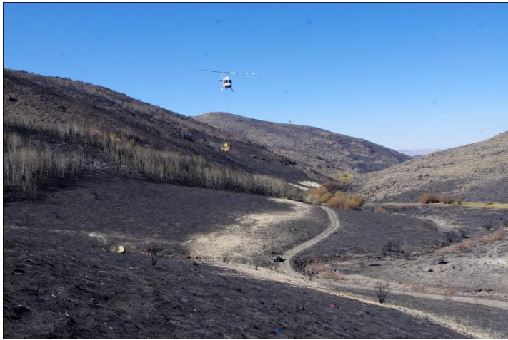
A helicopter spreads wood mulch on burned slopes above Willow Creek, to reduce erosion
